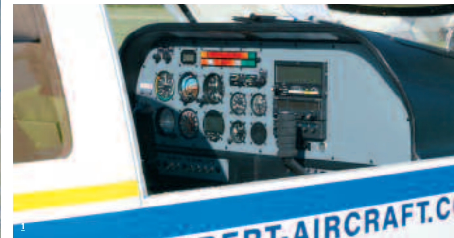
1 | The Mission's cockpit is light and airy, neat and tidy, with plenty of room on its wide panel. Production versions will have EFIS screens, electronic engine monitors and GPS moving map displays.
