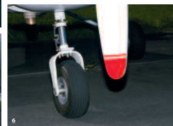
6 | Main gear legs are simple, tapering tubular steel springs, as yet unfaired, while the nose-leg is a lightweight gas strut, deliberately kept short to make it almost impossible to land nosewheel first, but still giving plenty of prop clearance.
