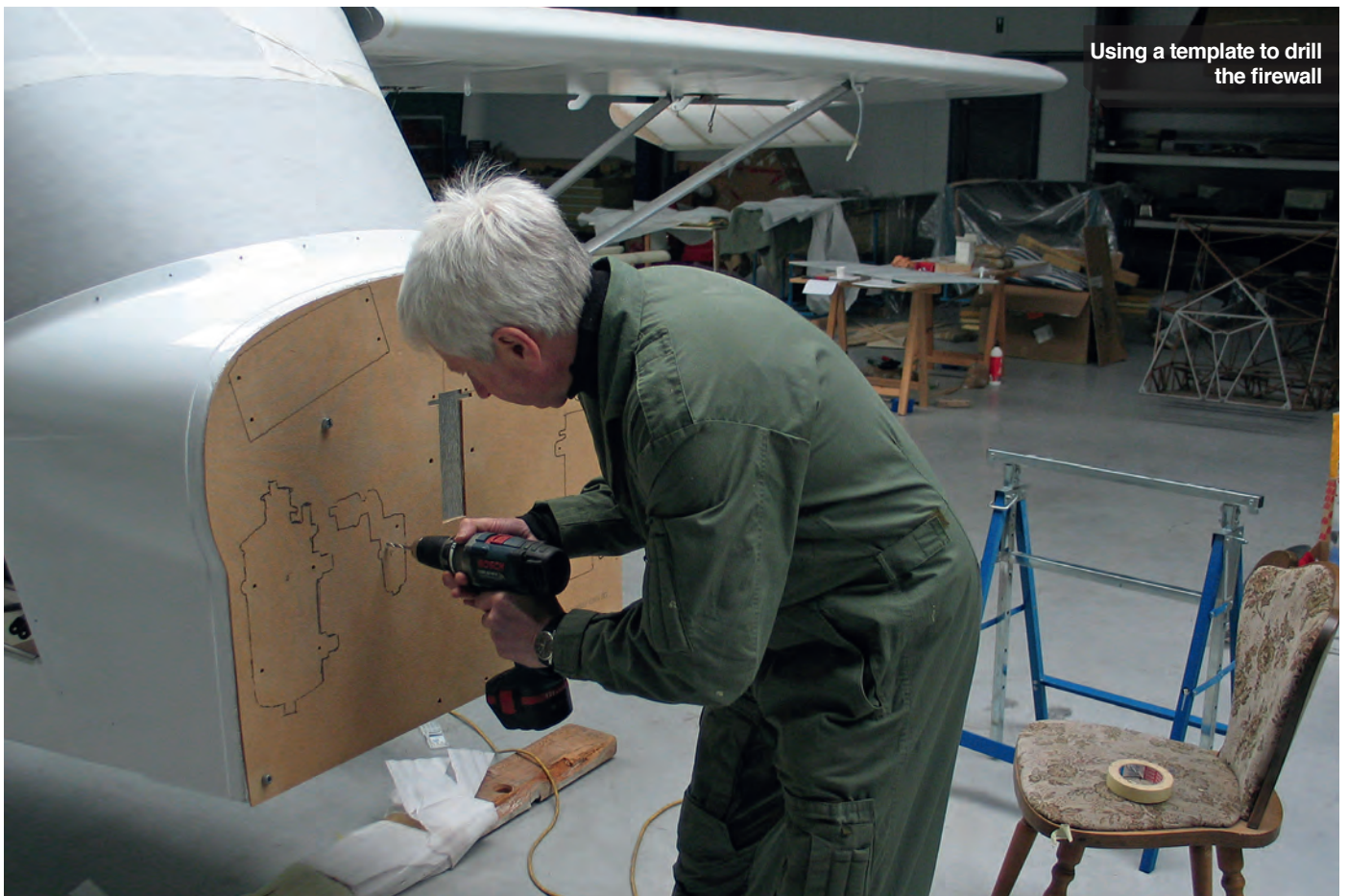
(Right) Fixing the heat shield to the firewall
