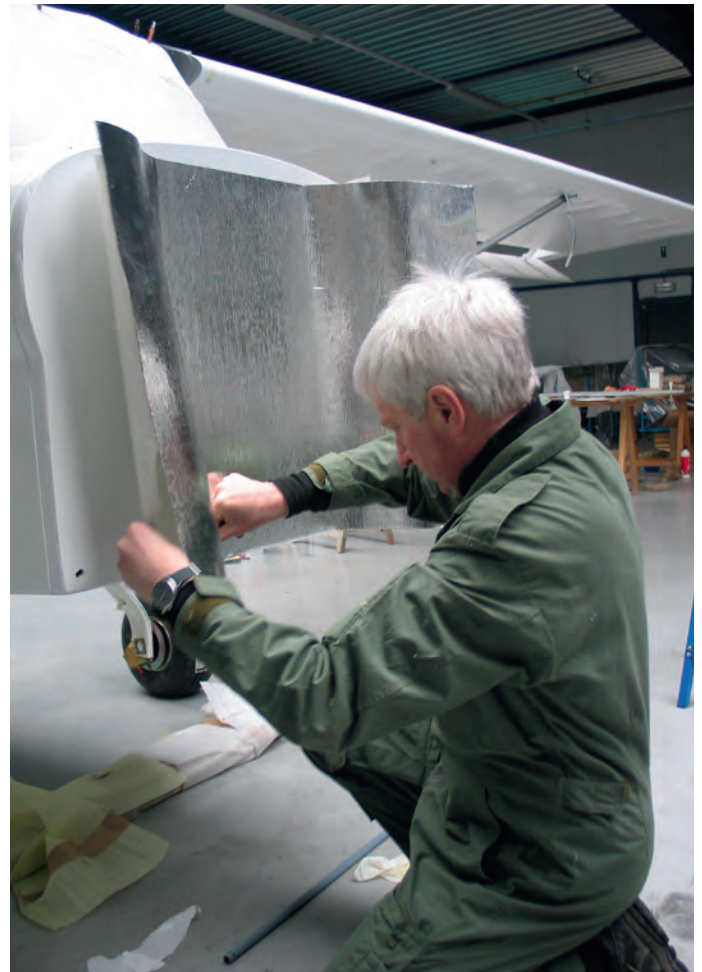
Using a template to drill the firewall
