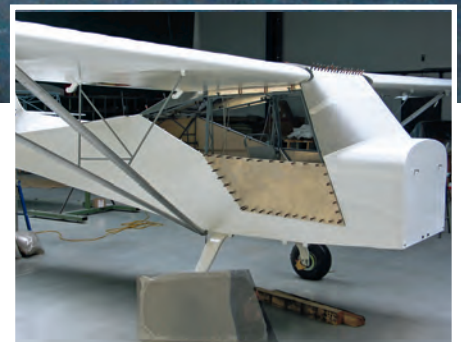
Cutting a transparent door window with a cutting disc – it worked better than I imagined it would
