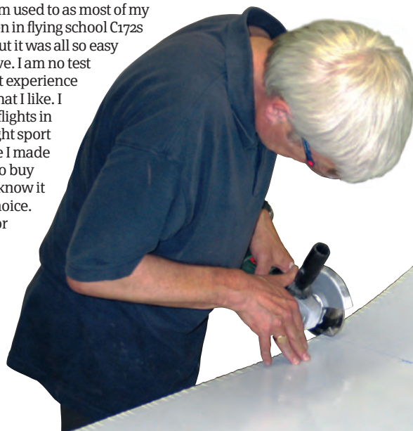
Cutting a transparent door window with a cutting disc – it worked better than I imagined it would
